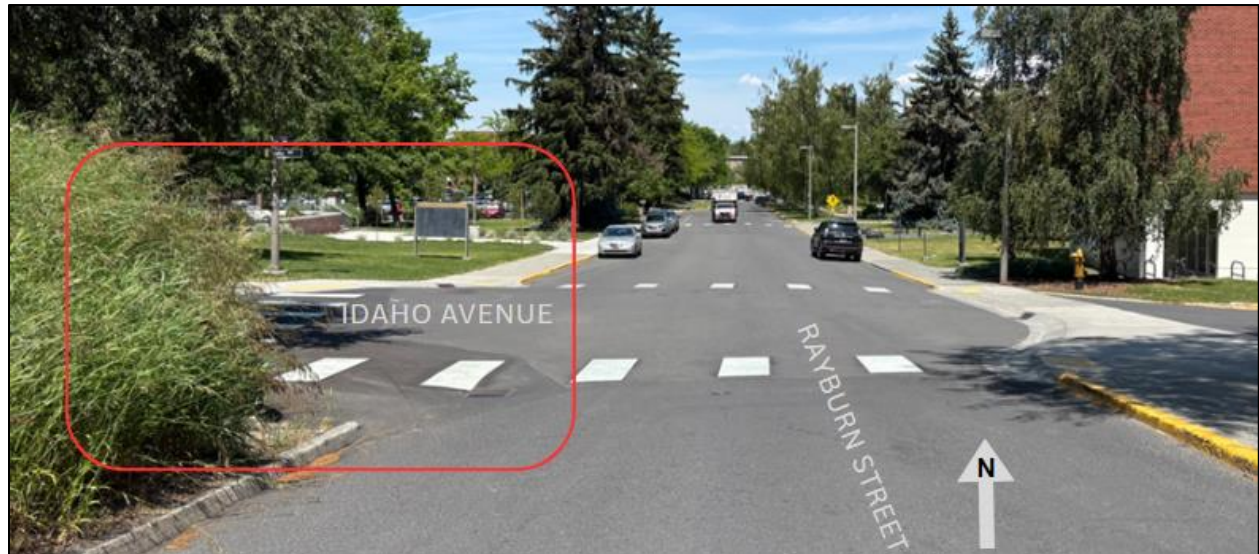
Crossing from northwest corner to southwest corner hide pedestrians from view of vehicles turning left onto Idaho Avenue
