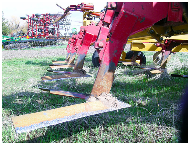
Figure 6.4. David Ostheller uses an undercutter (sweep) for post-harvest weed management. (Photo by Diana Roberts, WSU Extension.)
