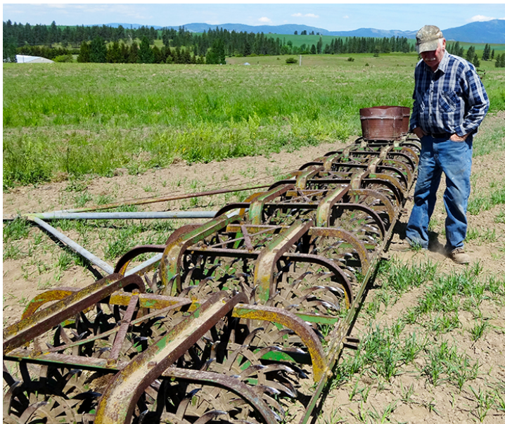
Figure 7.2. Ted Lacy's 50-ft rotary hoe consists of several units joined together. (Photo by Diana Roberts, WSU Extension.)
