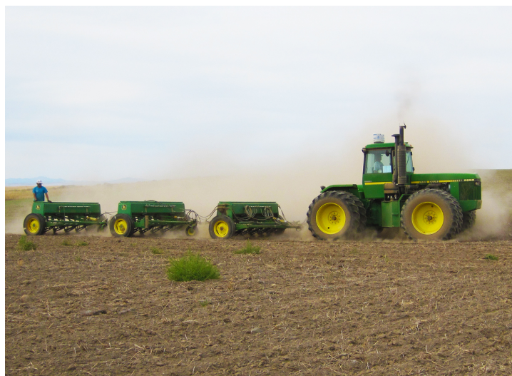
Figure 2.3. Running his 8300 Series John Deere drills in tandem enables Owen Jorgensen to put down seed and fertilizer in one pass. (Photo by Diana Roberts, WSU Extension.)
