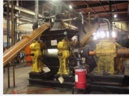
Multistage grinding to create ground/graded rubber
