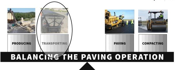
The synchronized balance of the four phases of asphalt paving to provide continuous paving operations.
