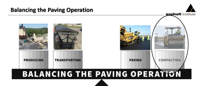
The synchronized balance of the four phases of asphalt paving to provide continuous paving operations.
