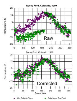
change in air mass (e.g., frontal passage). T<sub>dew</sub> may approach T<sub>min</sub> in arid and semiarid environments if nighttime winds are light
