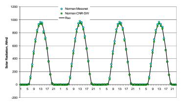
sensor followed the  $R_{so}$  curve relatively closely and the second sensor (CNR) averaged a few percent above the curve. Plots of  $R_s$  against the  $R_{so}$  curve also provides means to assess the accuracy of the datalogger clock, especially with older data sets.
